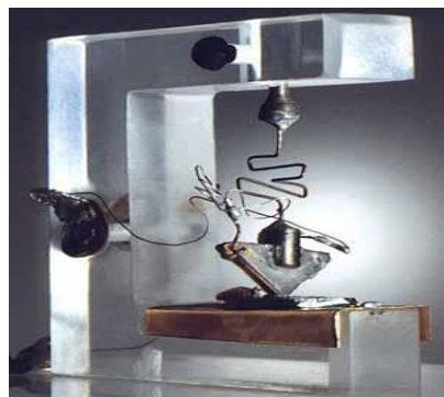
The First Working Transistor Bell Labs - 1947 Fig 4.9
